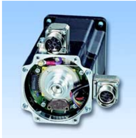
3-phase stepping motor with encoder (cover removed)
