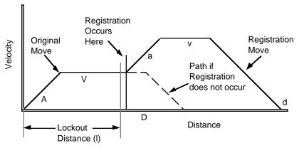
Registration is used to synchronize materials which slip or change size when processed.
