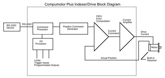
The current command to the amplifier is based on several quantities including the position of the servo motor's shaft, the desired position (which is generated by the indexer), and previous position errors.
