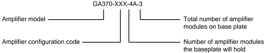
For this example each of the three amplifier modules would be labeled GA370-XXX with serial number. The 4 axes chassis would be labeled GA370-4A-3 with serial number.
