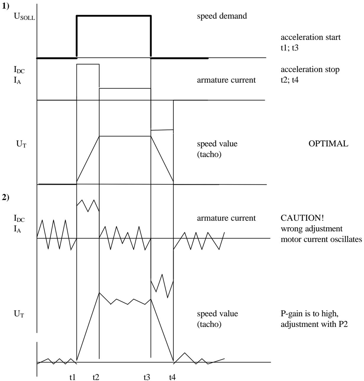
optimal adjustment of the speed controller - start-stop-operation
