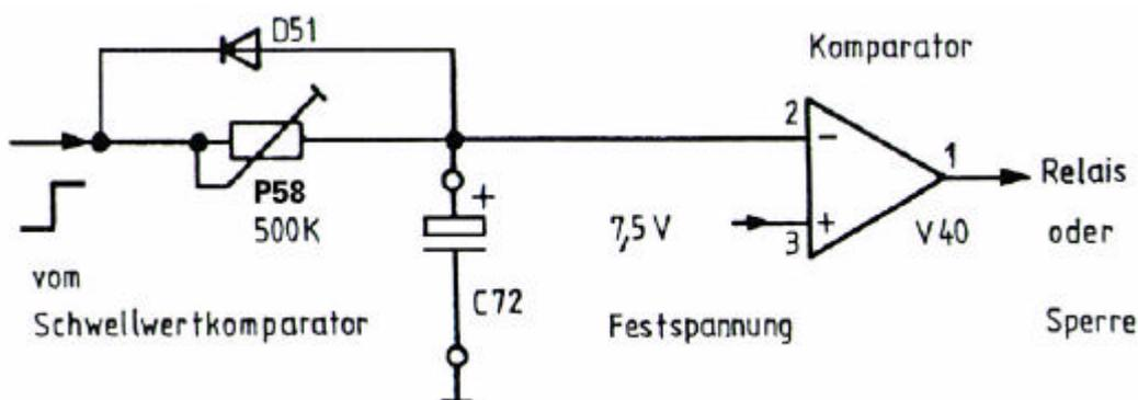
C72 is on soldering terminals and can be removed or modified if necessary.
