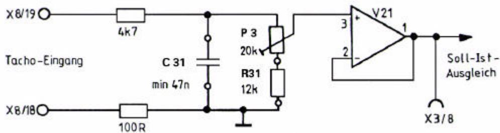
The range of input voltage can be extended by reduction of R31.
